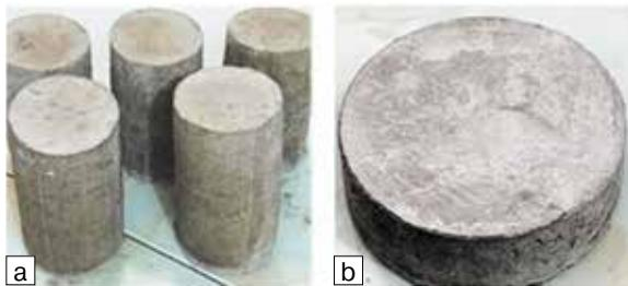
Figure 3. Concrete specimens for (a) compressive strength testing (b) abrasion testing. Photo A. W. R. Razzaq
