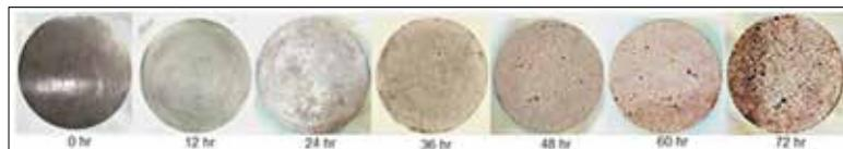
Figure 6. Various stages of abrasion on low strength polished concrete (LSPC) specimen. Author A. W. R. Razzaq
