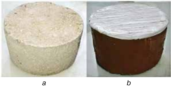
Illustration 2. Concrete disc (diameter 100 mm and height 50 mm) that was cut out from the cylindrical specimens. (a) Before coating. (b) After sealing the opposite side of the absorbing surface with plastic film and coating the remaining sides with epoxy resin. Author A. W. R. Razzaq
